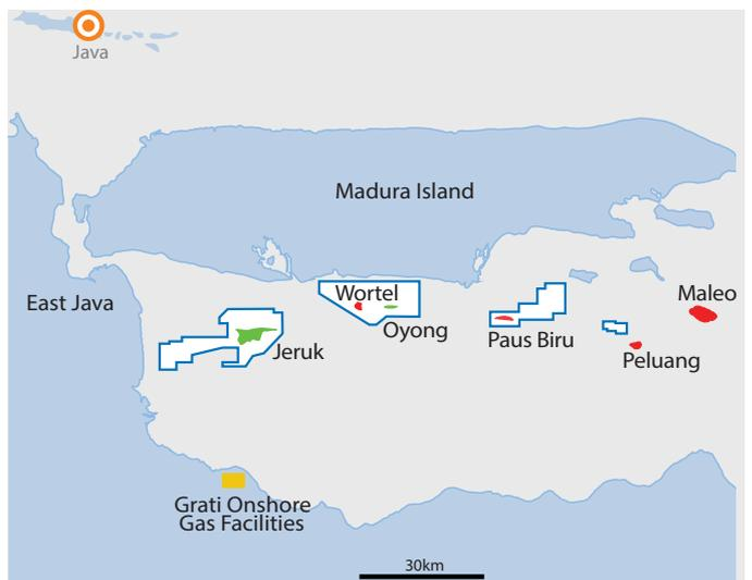
was approved subsequent to the end of the year. The approved POD consists of a single horizontal development well with an unmanned wellhead platform (WHP), connected by a subsea pipeline to the existing WHP at the Oyong field, approximately 27km away.
