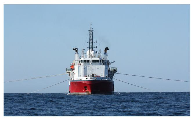
Voyager Explorer conducting the Pipeline 3D seismic survey in PEP 51313, Taranaki Basin, New Zealand (courtesy Seabird Exploration)
