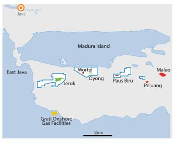
was approved subsequent to the end of the year. The approved POD consists of a single horizontal development well with an unmanned wellhead platform (WHP), connected by a subsea pipeline to the existing WHP at the Oyong field, approximately 27km away.
