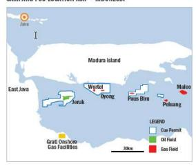
The Paus Biru development is planned to consist of a single well and wellhead platform at the Paus Biru gas field, with a 27km subsea pipeline connecting the well to existing infrastructure at the Oyong field. Subject to final approvals, gas production from Paus Biru is expected to commence by 2025 at a rate of 20-25 mmcfd.
