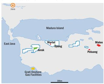
from a drill stem test (DST) over a 29 metre interval between 576 and 605 meters Measured Depth. Technical analysis following the discovery is ongoing in preparation for a Plan of Development to be submitted to the Government of Indonesia. The preliminary development plan is for a single well development with a pipeline to the existing Oyong infrastructure.
